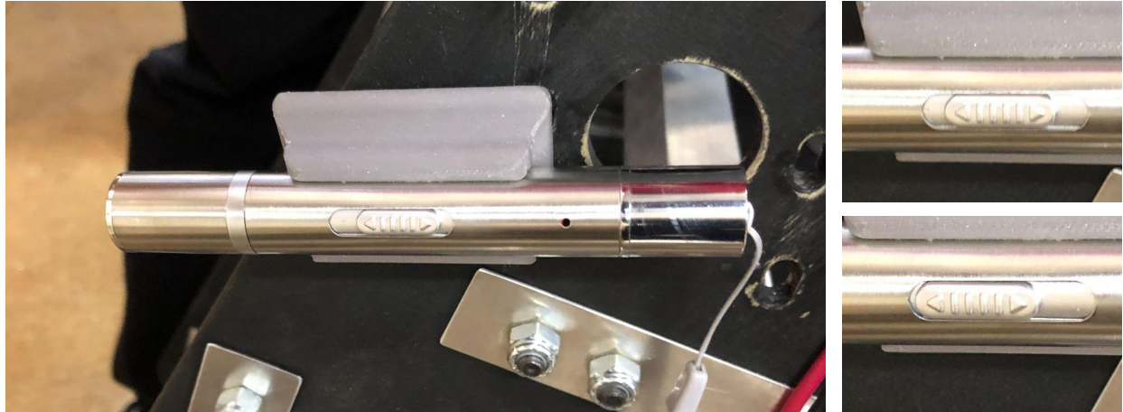
The laser pointer in the LASER, BLACK_LIGHT, and FLASHLIGHT modes respectively. Full right on the switch corresponds to OFF.
