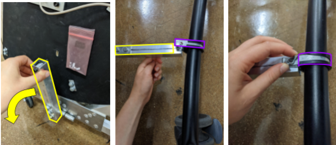
Processes of connecting an attachment bar to its bracket, with attachment bar outlined in yellow and bracket outlined in purple.
