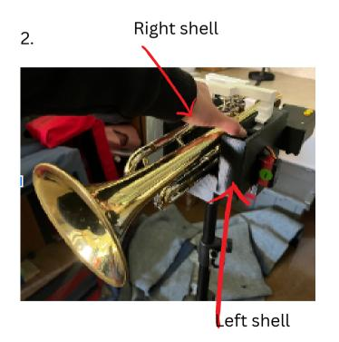
2. With one person supporting the trumpet, have another slide the left shell into the bottom of the trumpet and next to the right shell. Mate the two shells by sliding the left shell slot onto the bottom of the trumpet. You may need to lightly wiggle/shake the shells and valves so they seat together.
