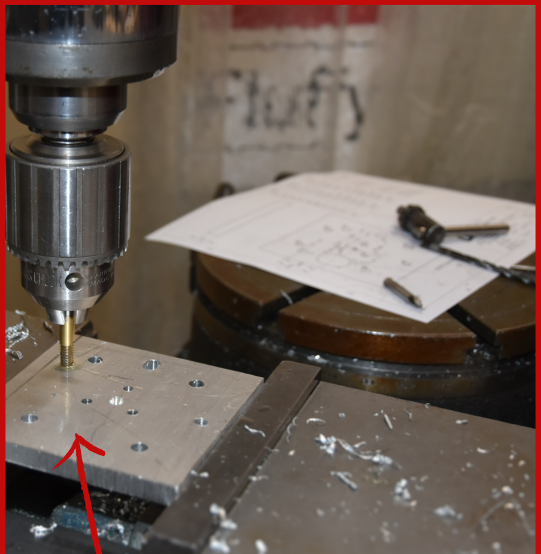
A gear hub being powertapped using a spiral point tap in a key chuck
